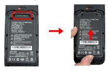
**4.** Press down the battery to secure in place.
