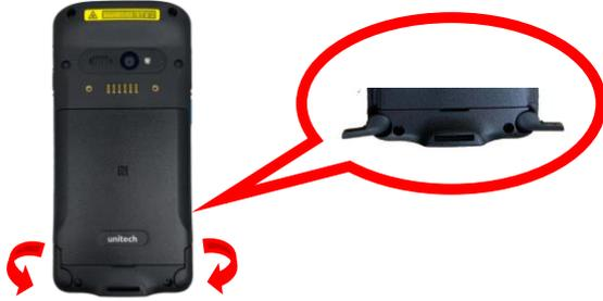
2. Pull the battery up to remove it.
