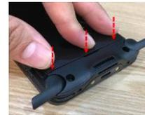
4. Lock the battery cover by turning the knobs a quarter of a turn (90°). Make sure the battery cover is securely closed, or you may be unable to turn on the terminal.
