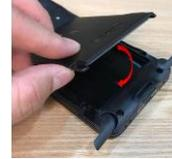
3. Align the batter cover with the recesses of the battery compartment, and press the battery cover down to secure in place. Make sure there is no gap between the device and the battery cover.
