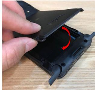
3. Press the battery cover down to secure in place. Make sure there is no gap between the device and the battery cover.
