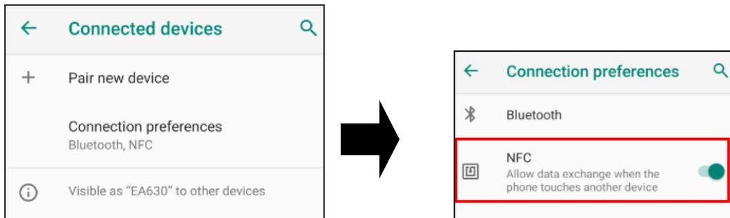
3. Make sure that both devices are unlocked and have NFC turned on. Also make sure that the NFC antenna area of EA630 and the other phone's NFC area are close to one another. Slightly moving the phones until a connection is made. Tap the screen.
